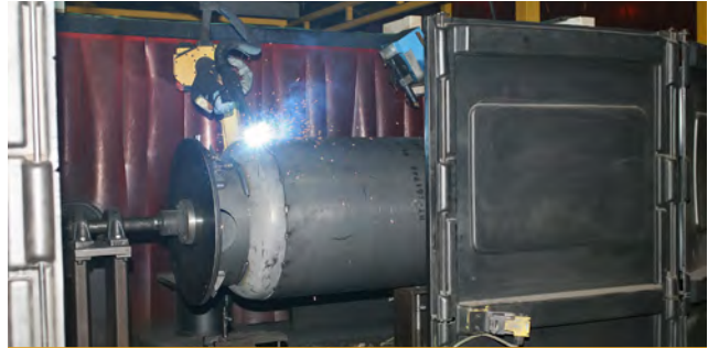
Of the 11 robotic welders at Mi-T-M, one is dedicated to welding air compressor vessels
