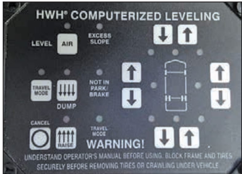
Figure 15-7: Leveling system control panel
