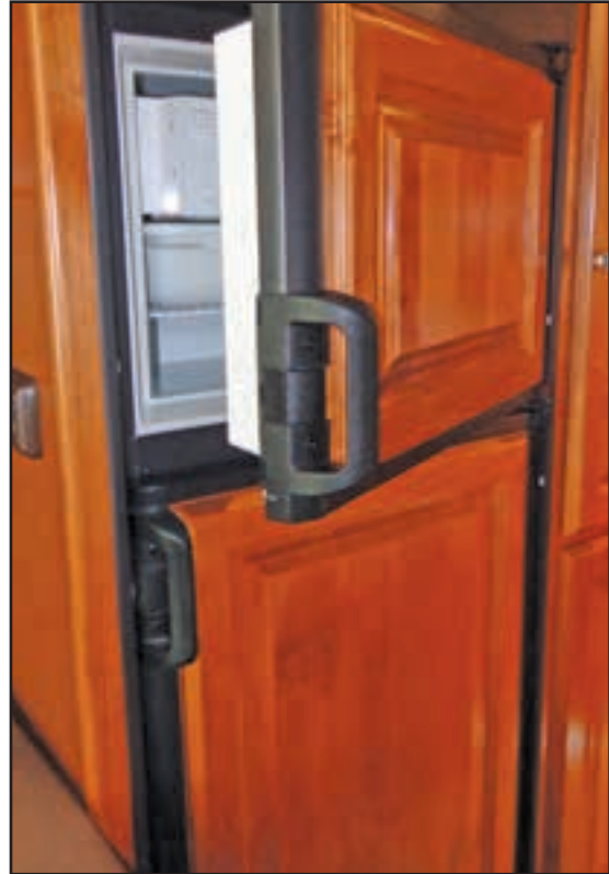
Figure 5-1: Standard LP/ Gas Refrigerator
