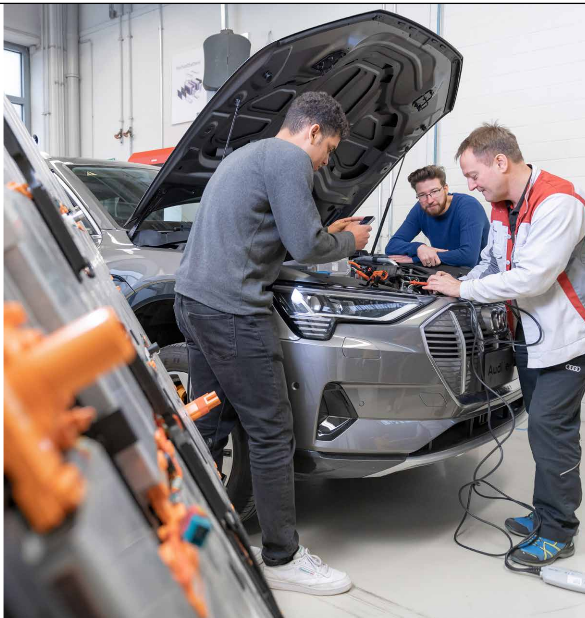
Trainer Rupert Kaindl explains to Audi employees Felix Fornoff and Leon Meka (from right) how the Audi e-tron* is disconnected from the battery.
