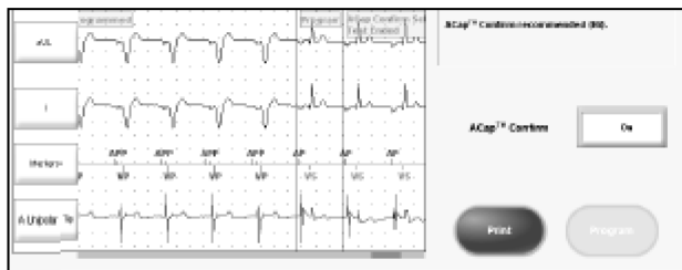
Figure 7. ACap™ Confirm Setup test results window in the Zephyr DR device
