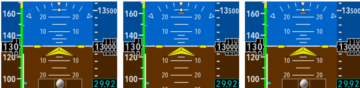
Figure 4-12 KI 300 Slip/Skid Indicator Display Options
