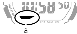
a. Control indicator
