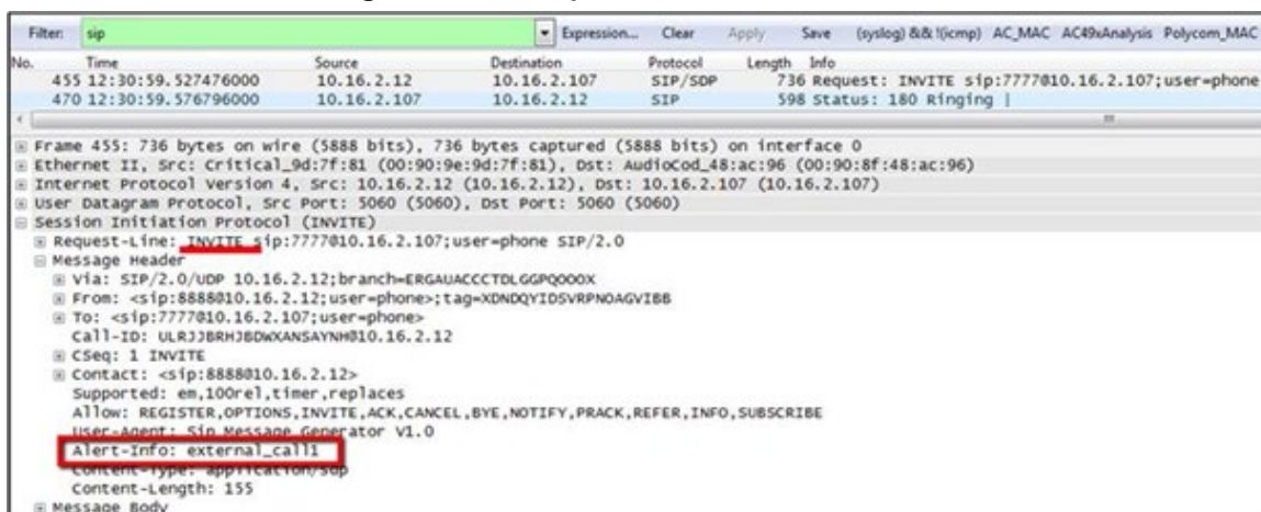
Figure 5-2: Example of the Alert-Info Header
