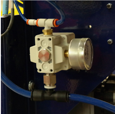
5/32" tubing to blocking valve 1/4" tubing to cylinder
