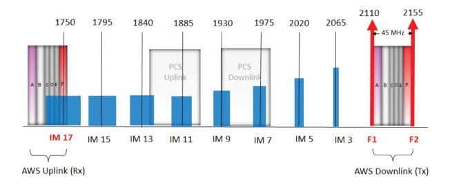
Problems can occur, however, when AWS spectrum is combined with PCS spectrum in a common feed system. In this scenario it is possible for IM3 to fall in the AWS uplink band and negatively impact site performance.
