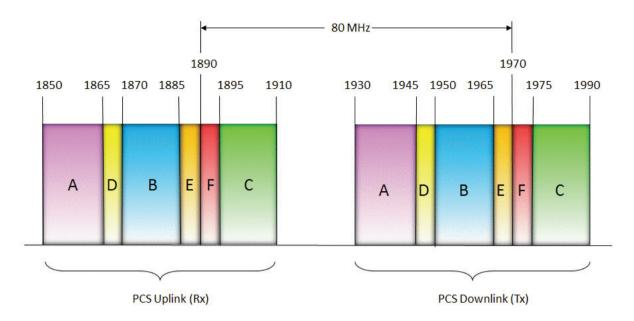
The FCC did a good job when designing the PCS spectrum in that the lowest order PIM product that can fall in a single spectrum owner's uplink band is IM11. This means that individual blocks of PCS spectrum are fairly robust against intermodulation interference. PIM sources that might cripple the performance of 700 MHz or 850 MHz systems (which allow IM3, IM5 or IM7 signals to fall in-band) may not severely impact PCS band performance.
