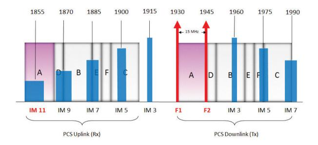
Problems can occur, however, when multiple blocks of PCS spectrum are co-located on the same antenna system. This can happen when an operator acquires additional PCS licenses in a given market or when multiple PCS operators share a neutral host DAS. In this scenario, it is not uncommon for IM3 or IM5 to fall in band and generate harmful interference for one or more PCS operators.
