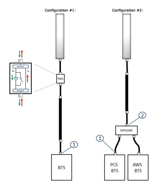
Site configuration #1 shows a single band system with a Tower Mounted Amplifier (TMA) installed at the top of the tower. If this were a PCS band system two PCS test tones could be injected at point #1 to fully test this site. The two PCS band test tones (F1, F2) are able to pass completely through the system and out the antenna. Any PIM generated along the path can pass directly back to the test set for analysis.
