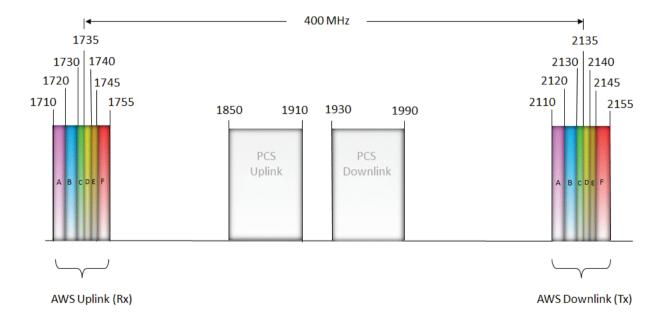
Due to the extremely wide separation between AWS band uplink and downlink frequencies it is highly unlikely for AWS downlink signals by themselves to generate PIM at a level that will impact system performance. The lowest order PIM product that can fall in a single AWS operator's own uplink band is IM79! Even when multiple blocks of AWS spectrum are combined together in a common feed system the lowest order PIM product that can fall in the AWS uplink band is IM17.
