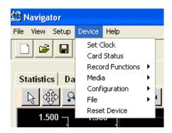
The remote recorder can be controlled from the **Device** Menu. As shown at left, the user can set the clock, get the card status (Compact Flash card in the remote recorder), Control the record functions, Change the Recorder configuration, manipulate files and reset the device. Note that a number of these functions cannot execute if the remote recorder is in record mode or the real time graphing is active. You will receive warning messages.
