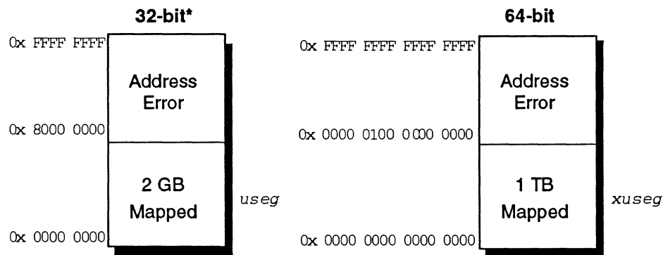
Figure 3-4 User Mode Virtual Address Space
