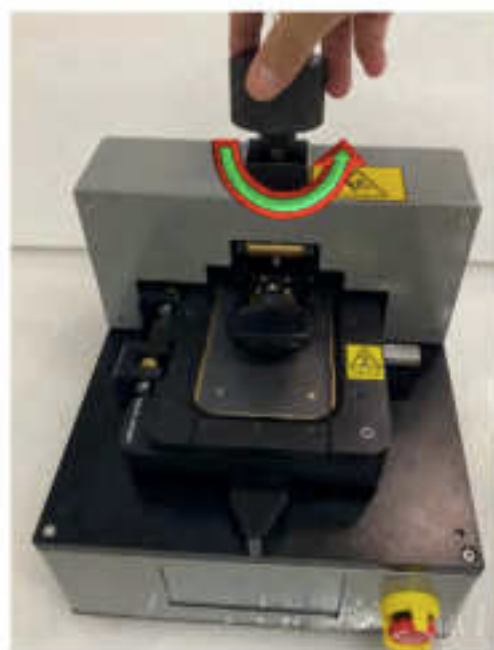
Turn the knob counterclockwise until the screen is pulled up to remove the screen
