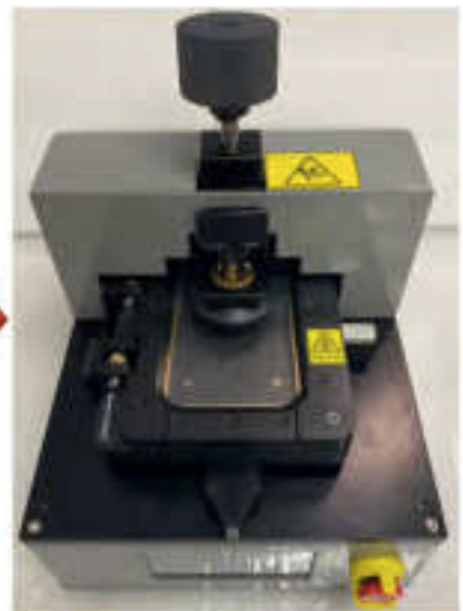
Hot Pocket full insert RFID automatic identification model and power on. The Hot Pocket starts heating from room temperature to the specified temperature, and starts counting down 120s after reaching the specified temperature
