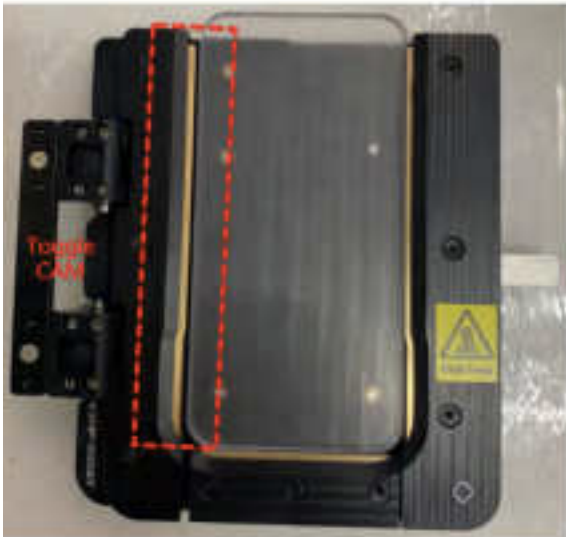
There is a gap between the West Bar and the phone when not clamped
