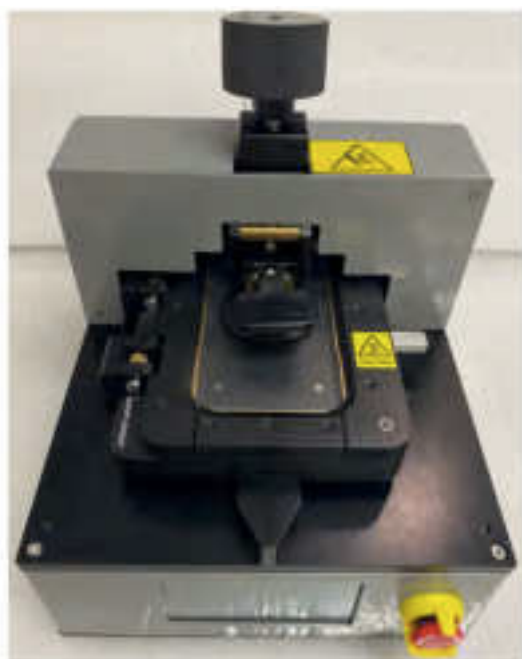
After pressing the suction cup OK, the screen can begin to remove, and the display begins to count down for 15 minutes
