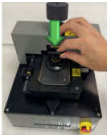
Turn the handle of the suction cup downward 90° to ensure that the suction cup is firmly attached to the surface of the phone.
