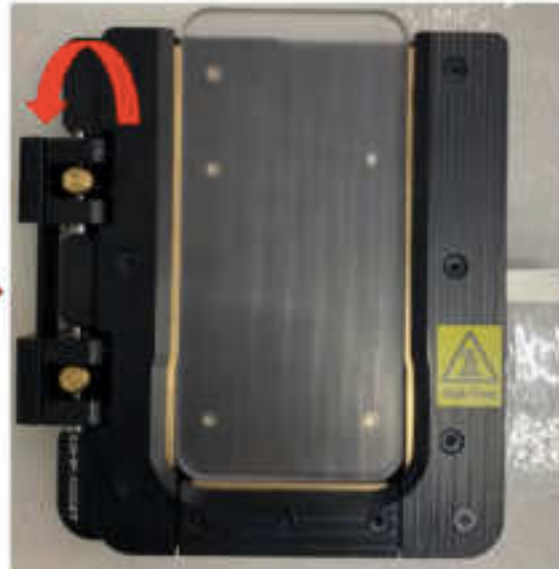
Flip down Toggle CAM 90° to make the West Bar fully fit with the mobile phone to complete clamping
