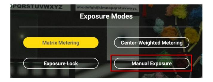
Step 3. Users can press the **Manual Exposure** button which is shown as the above diagram for setting the Shutter and Gain manually.
