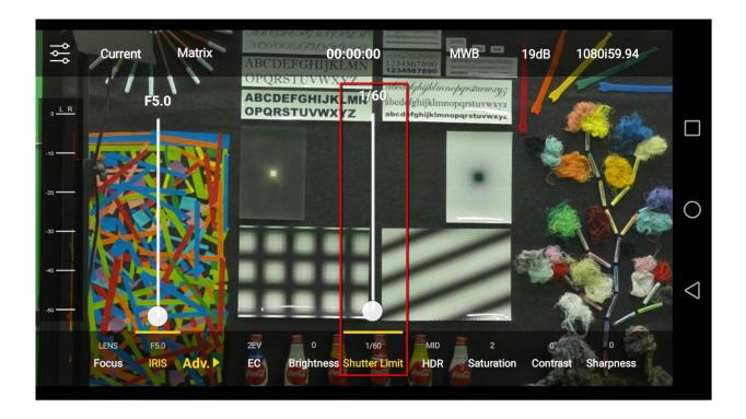
Step 5. In the Manual Exposure Mode, please press the 19dB option which is shown as following diagram to enter the Gain Limit option to adjust the Gain Limit manually by the Gain Limit slider.
