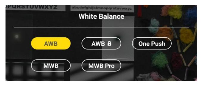
MWB: Users can press the MWB button to adjust the desired White Balance color temperature by the slider which is shown as the following diagram. The adjustable color temperature range is 2500K to 10000K.
