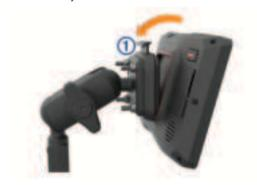
2 Push the top of the device forward until it snaps into place. The latch ① on the mount stays up after you insert the device.
