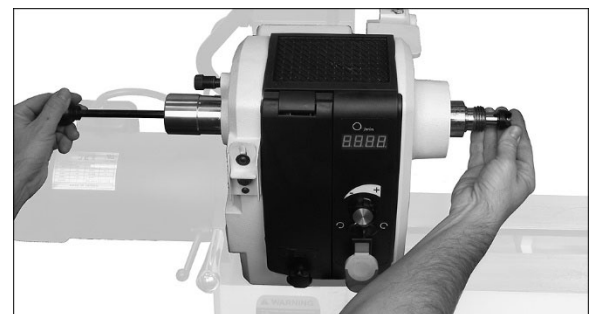
Figure 7-8: removing spur center
