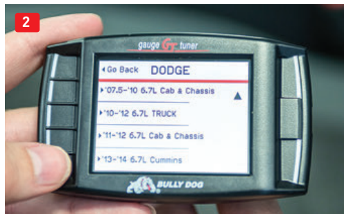
(1) Cable harness that comes with the tuner is first plugged into the OBDII port for the initial programming. (2) Monitor screen is used to select year, vehicle and engine. Touch buttons on each side of screen are used while following specific prompts that make programming effortless. (3) A special cable harness is used to unlock the Ram PCM and must only be used for this step. Red flag distinguishes the cable from the one in the kit.
