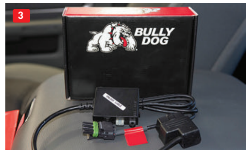
(1) Cable harness that comes with the tuner is first plugged into the OBDII port for the initial programming. (2) Monitor screen is used to select year, vehicle and engine. Touch buttons on each side of screen are used while following specific prompts that make programming effortless. (3) A special cable harness is used to unlock the Ram PCM and must only be used for this step. Red flag distinguishes the cable from the one in the kit.
