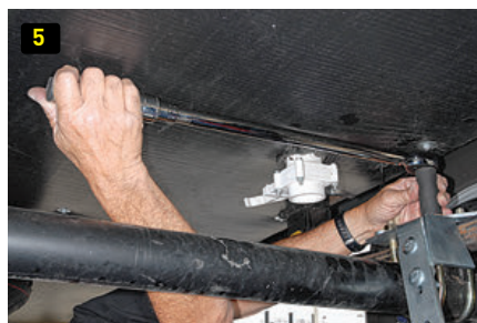
(3) Remove the two factory U-bolts and set aside for later use, but discard the factory tie plate. (4) Install the Joy Rider shock mount assembly utilizing the factory U-bolts and the supplied stiffener plates — two per shock plate assembly. (5) Use an alternating cross pattern with an accurate torque wrench to tighten the U-bolts to 90 ft-lbs. (6) Loosely bolt the Joy Rider shock absorber to the shock mount extension to aid in installing the upper bracket to the optimal position.
