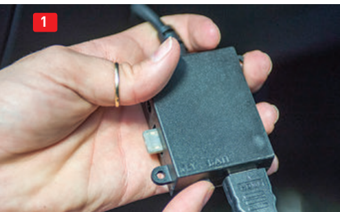
(1) Cable harness that comes with the tuner is first plugged into the OBDII port for the initial programming. (2) Monitor screen is used to select year, vehicle and engine. Touch buttons on each side of screen are used while following specific prompts that make programming effortless. (3) A special cable harness is used to unlock the Ram PCM and must only be used for this step. Red flag distinguishes the cable from the one in the kit.
