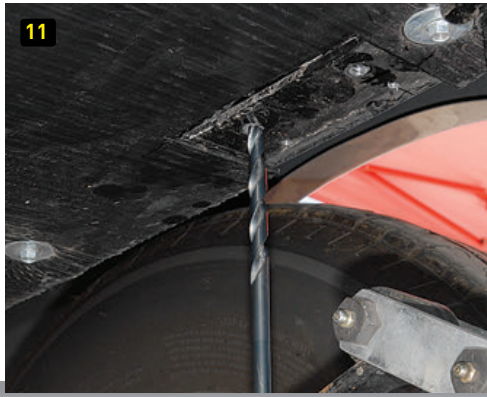
(10) A cordless impact wrench will be invaluable when installing the Joy Rider shock absorber to the upper and lower brackets. (11) Using a 12-inch-long drill bit will allow for adequate reach when installing the upper bracket because the leaf springs will be in the way of a drill with a shorter bit. (12) When installing the 3/8-inch self-drilling bolts to the upper bracket, the cordless impact wrench came in handy when equipped with an 8-inch 1/2-inch drive extension and 3/16-inch-deep socket.
