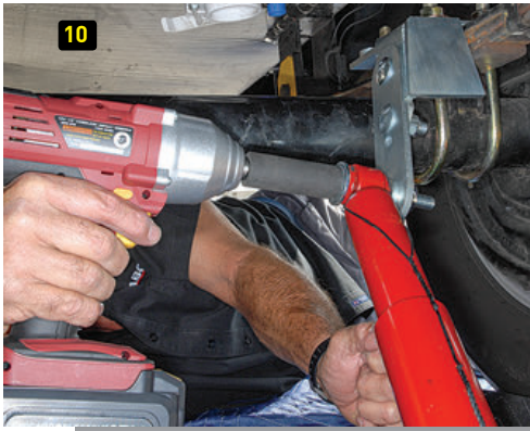
(10) A cordless impact wrench will be invaluable when installing the Joy Rider shock absorber to the upper and lower brackets. (11) Using a 12-inch-long drill bit will allow for adequate reach when installing the upper bracket because the leaf springs will be in the way of a drill with a shorter bit. (12) When installing the 3/8-inch self-drilling bolts to the upper bracket, the cordless impact wrench came in handy when equipped with an 8-inch 1/2-inch drive extension and 3/16-inch-deep socket.
