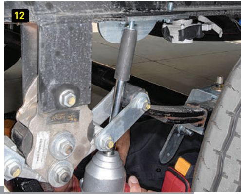
(10) A cordless impact wrench will be invaluable when installing the Joy Rider shock absorber to the upper and lower brackets. (11) Using a 12-inch-long drill bit will allow for adequate reach when installing the upper bracket because the leaf springs will be in the way of a drill with a shorter bit. (12) When installing the 3/8-inch self-drilling bolts to the upper bracket, the cordless impact wrench came in handy when equipped with an 8-inch 1/2-inch drive extension and 3/16-inch-deep socket.
