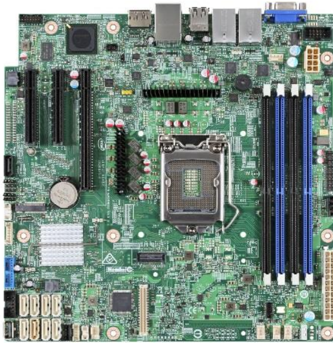
Figure 1. Intel® Server Board S1200SP Layout (S1200SPL)
