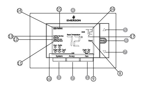
Whenever "peplace" appears in the display, new premium brand AA alkaline batteries should be installed. If the house will be unoccupied for an extended period and either "or "peplace" is displayed, install new batteries before leaving.
