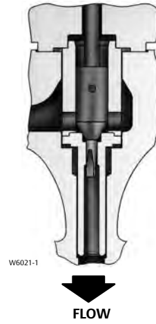
Figure 14. Fisher HPAS Trim with Micro-Flat Valve Plug
