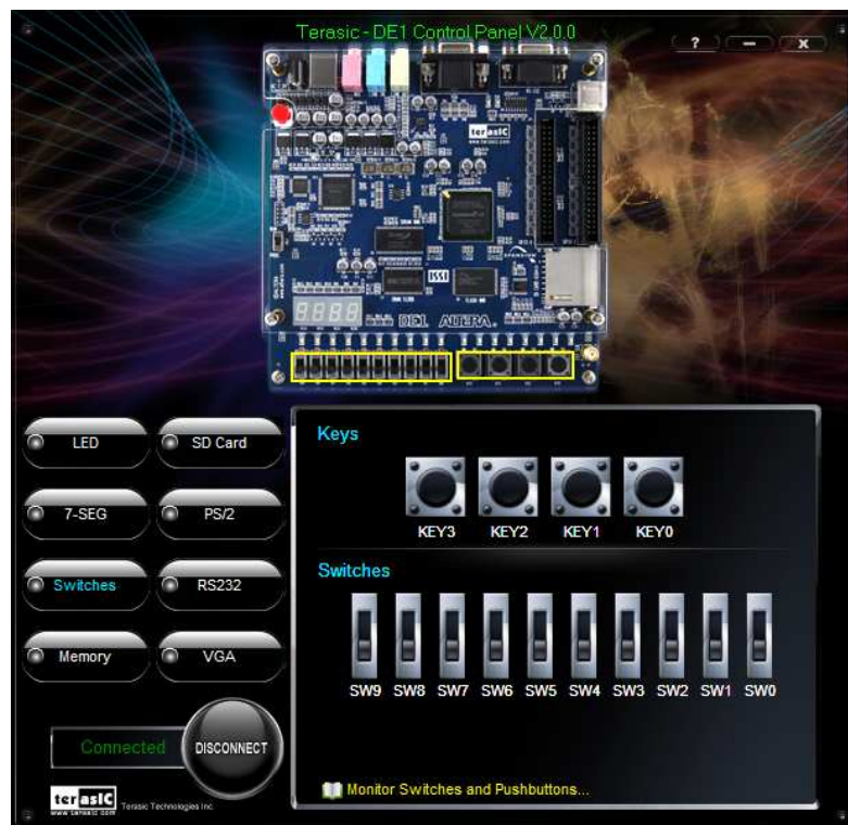
Figure 3.5. Monitoring switches and buttons.
