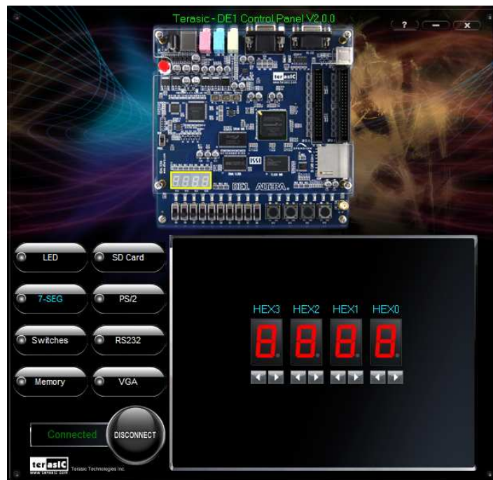
Figure 3.4. Controlling 7-SEG display.
