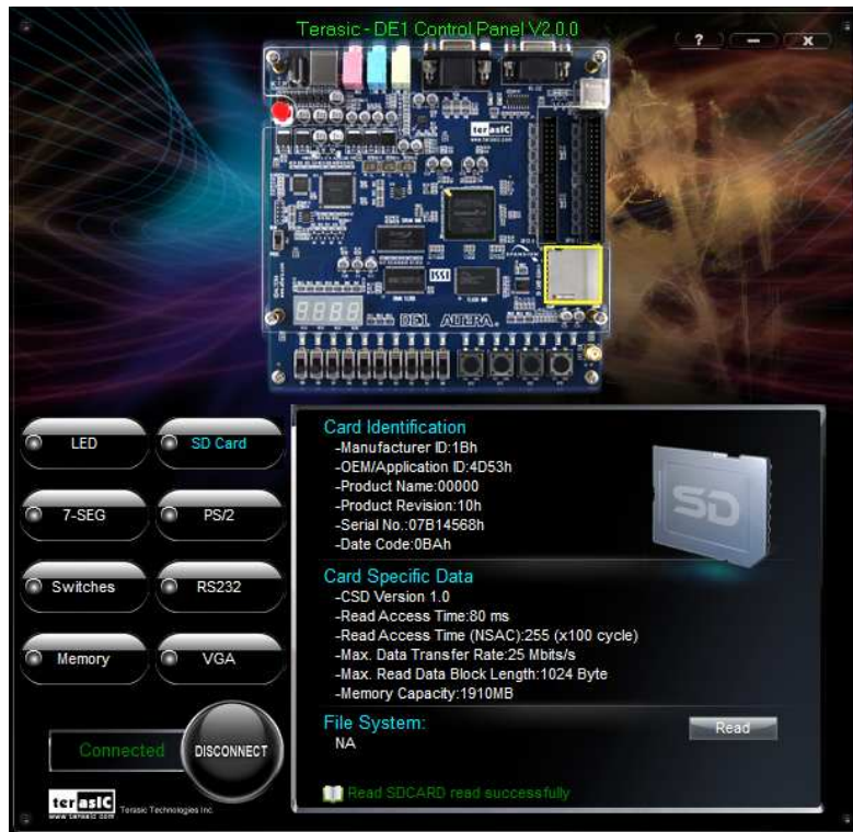
Figure 3.8. Reading the SD Card Identification and Specification.
