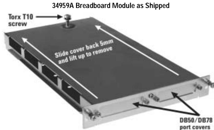
The Agilent-supplied PC board must be removed if you are making connections to the Analog Buses, in order to solder the necessary relays (not provided) and lead wires. To remove this PC board, remove the Torx T10 screw shown, slide the cover back 5mm to clear the two retaining tabs, and lift the board up. Reverse this procedure to reinstall the board.
