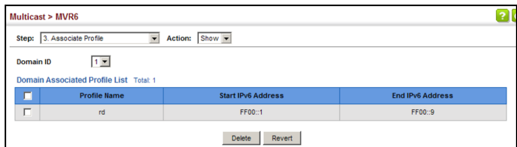
Figure 384: Showing MVR6 Group Address Profiles Assigned to a Domain
