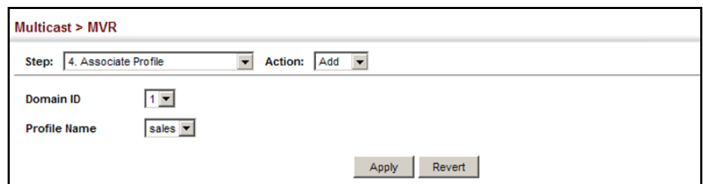
Figure 370: Assigning an MVR Group Address Profile to a Domain
