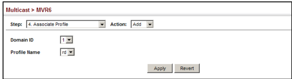
Figure 383: Assigning an MVR6 Group Address Profile to a Domain
