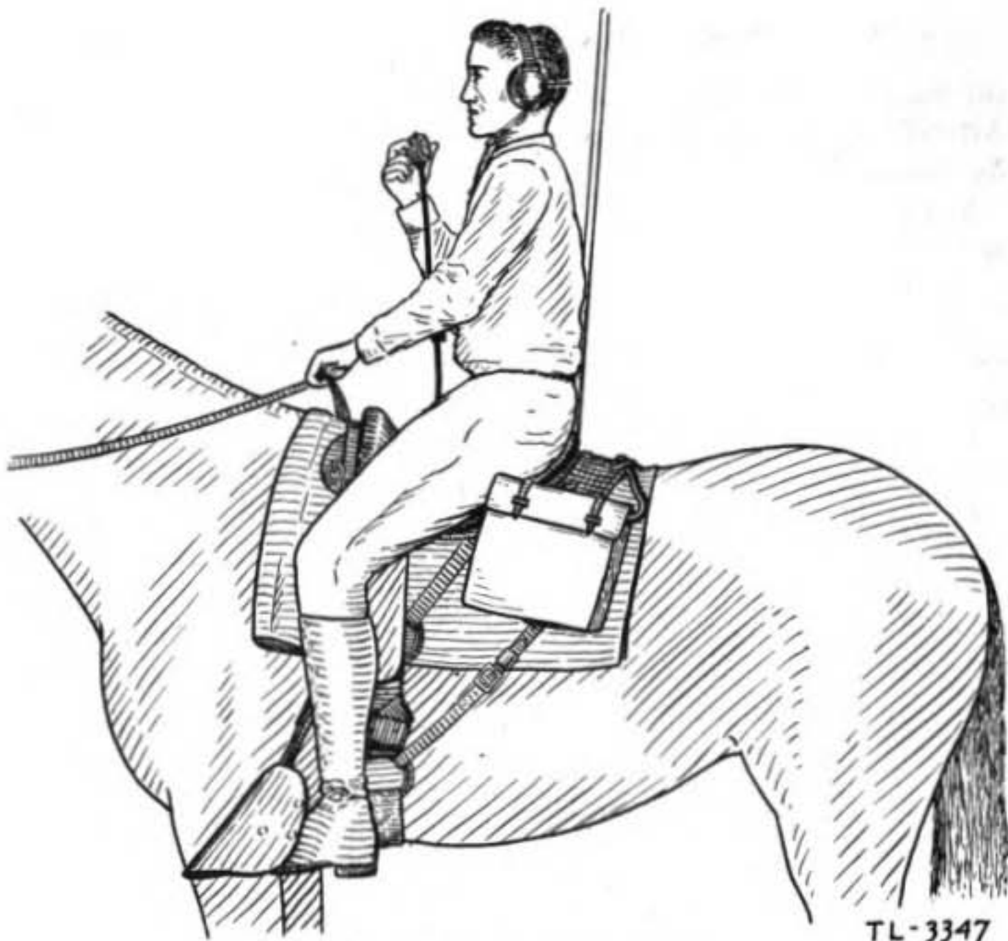
① Near side, showing battery pocket.
