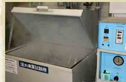
Plated hardware being subjected to corrosive salt spray
