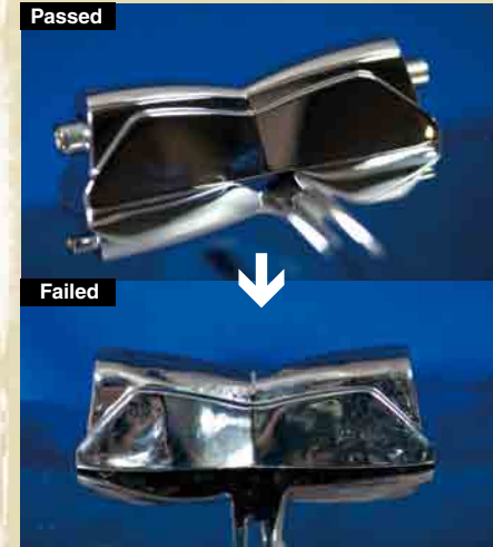
The results of a plating heat resistance test
