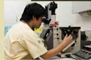
Microscopic examination of plating thickness and quality
