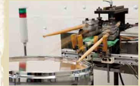
Extended durability tests ensure that our drums will stand up to heavy use
