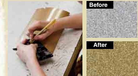
Cutting finishes to test adhesion
