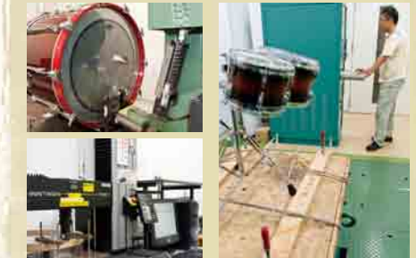
Products are subjected to extreme heat, cold, and humidity in accelerated environmental testing chambers
