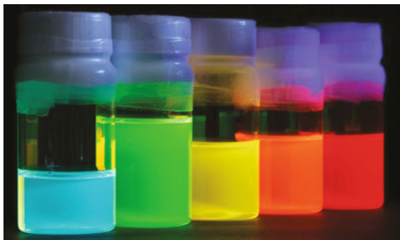
Fig. 2.1 Luminescence from suspensions of colloidal CdSe nanocrystals (1.7–4.5 nm diameter, from left to right ) under UV excitation ( courtesy A. Brinkman and M. Vis, Utrecht University)
