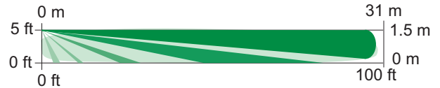
Side View Optional Long Range Coverage: 30.5 m x 3 m (100 ft x 10 ft) Requires optional ORL92-3 lens.
