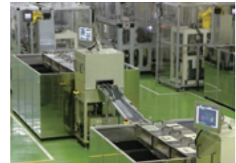
Ink cartridge recycling equipment
