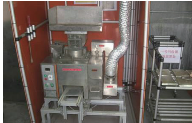
Solder recovery machine
