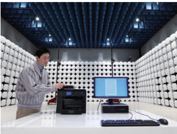
EMI measurement of products in an anechoic chamber
