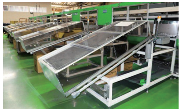
Automated toner cartridge sorting system
