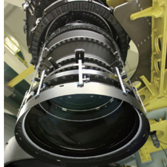
Wide field corrector installed in the HSC
