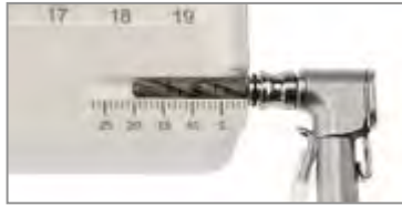
With The Mount On The Drill, Measure From The Tip Of The Drill To The Mount
