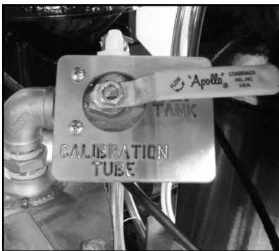
Pump #1 pumping liquid into the top of the mix tank when Seed Treatment Valve is in Calibrate.
