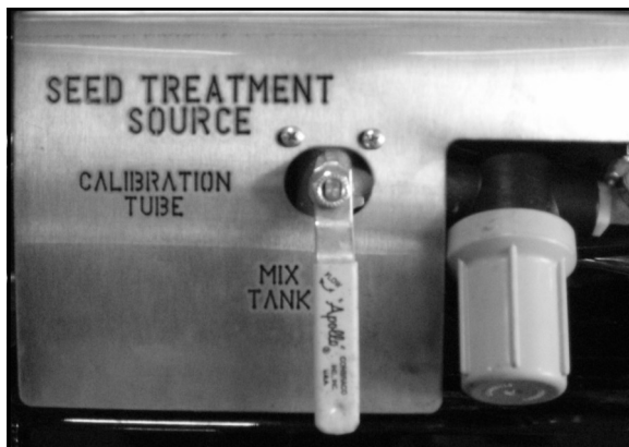
Pump #1 Drawing from bottom of Mix Tank
