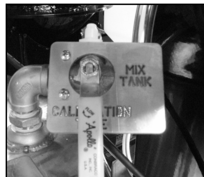
Pump #1 pumping liquid into the top of the calibration tube when Seed Treatment Valve is in Calibrate.
