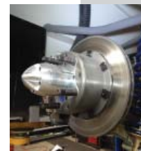
4-1/2" to 3" Brake duct adapter - no fan.
