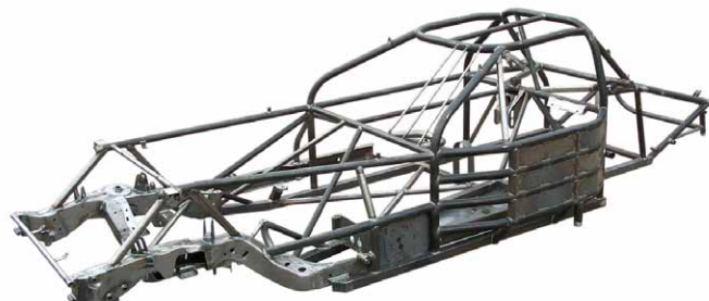
Modified Chassis with Impala Frame
