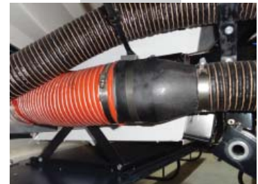
4-1/2" to 3" Brake duct adapter - no fan.
