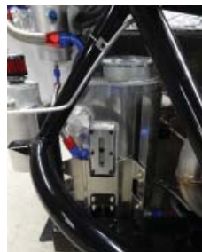
A 10 quart Howe oil tank includes a sight glass for checking oil level at a glance
