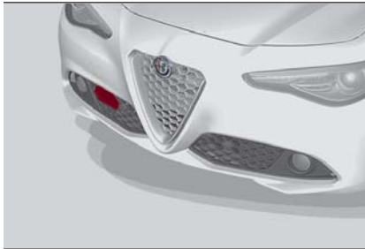
Front Bumper Radar Location
