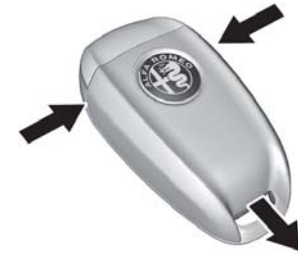
Emergency Key Release Buttons
