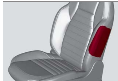
Front Supplemental Seat-Mounted Side Air Bag
