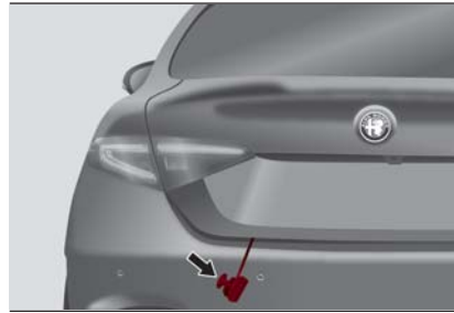
Manual Release Cord Shown With Trunk Closed
