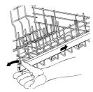
Version B: with adjustment in three positions on both sides.
