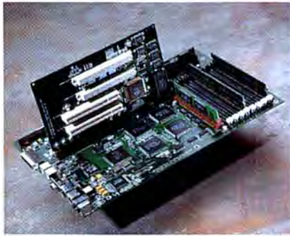
The $249 riser card adds NuBus slots to the new Power Computing PowerWave 604 systems.
