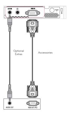
You can connect the audio cable without using a gender as shown in the illustration above.
