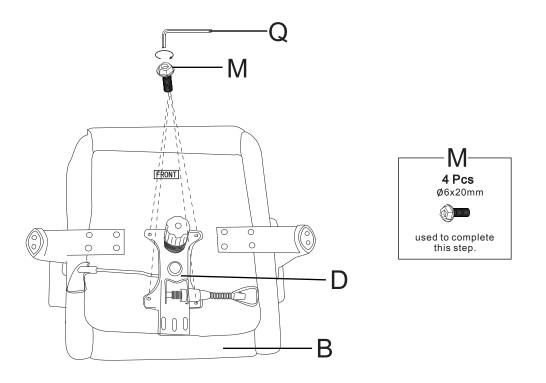
Note: Align the Seat Plate (D) so the FRONT of the Seat Plate matches the FRONT label on the bottom of the Seat Cushion (B). Tighten the screws with Allen Key (Q).
