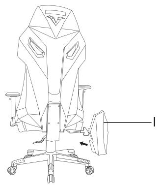
Note: Fasten the decorative buckle (I) by pushing until connect is secure.
