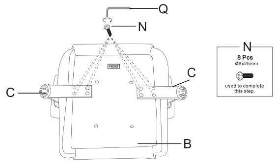
Note: Attach Armrests (C) to the Seat Cushion (B) using 8 x Screws (N) with Allen Key (Q). Tighten the screws with Allen Key (Q).
