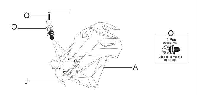
Note: Attach BackBar (J) to the Back (A) using 4x Screw(O) with Allen Key (Q). Tighten the screws.
