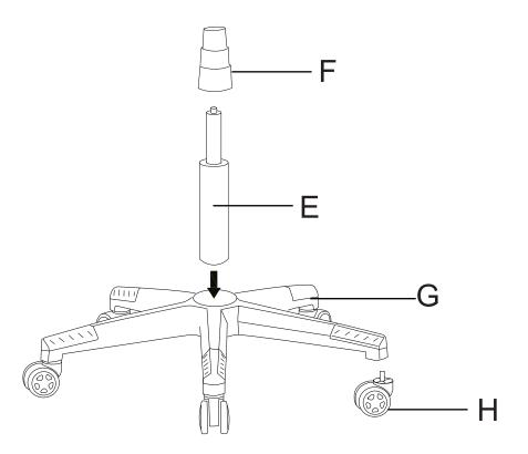
Note: Turn the Star Base (G) upside down. Push the Castors (H) into holes at the end of each leg. Turn the Star Base (G) upright and insert Gas Lift (E) into the center hole of Star Base (G). Place cover (F) over the Gas Lift (E).
