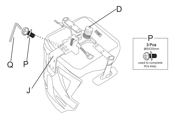
Note:Attach BackBar (J) to the mechanism (D) on the assembled Seat Cushion (B) using 3x Screw (P) with Allen Key (Q). Tighten the screws.
