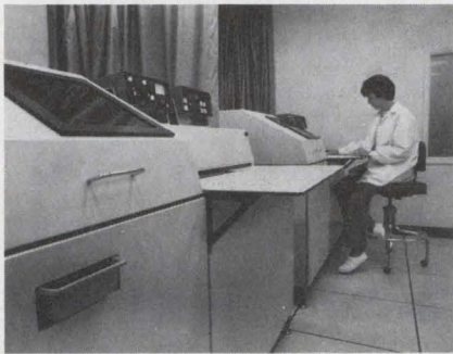
Beckman-designed machine-controlled laser trimmer can trim up to 20,000 resistors per hour. Laser trimmers are particularly effective in today's small geometry microcircuits.
