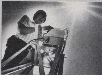
Gallium-arsenide solar cell only 1 cm in diameter can produce up to 10 W of electrical power.
