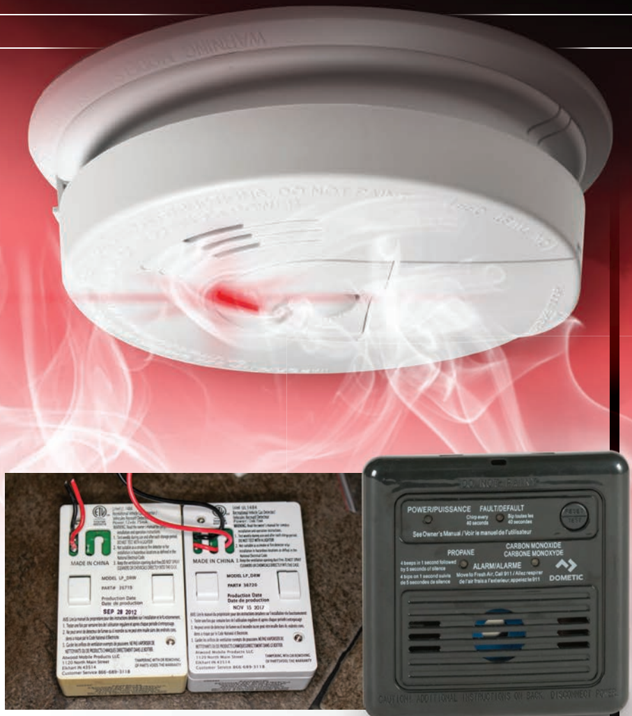
Above, left: Shown are the backs of the old and new Dometic/Atwood LP-gas detectors. Note the production date stamp. This detector will produce an alarm when it has reached its end of life, which is being powered for seven years. Above, right: Dometic also offers a 12-volt DC combination LP-gas and CO alarm for RVs.
