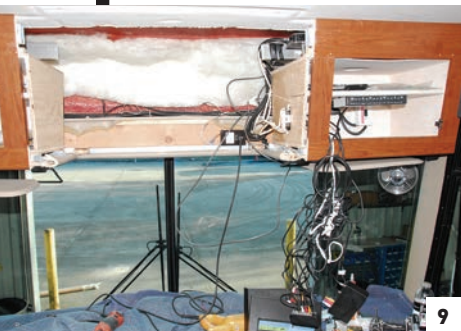
[9] With the TV and its metal structure out of the way, all of the excess wiring is removed, including the old RGB connections, digital converter and converter box wiring. [10] Here, the right-hand cabinet is shown with the excess wiring removed and necessary equipment remounted. [11] Dave and LJ's makes nearly everything needed for each job in-house. Here, a reinforcement bracket that will mount inside the cabinet and support the TV is fabricated.
