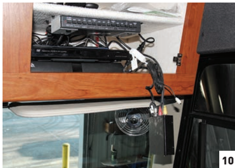
[9] With the TV and its metal structure out of the way, all of the excess wiring is removed, including the old RGB connections, digital converter and converter box wiring. [10] Here, the right-hand cabinet is shown with the excess wiring removed and necessary equipment remounted. [11] Dave and LJ's makes nearly everything needed for each job in-house. Here, a reinforcement bracket that will mount inside the cabinet and support the TV is fabricated.
