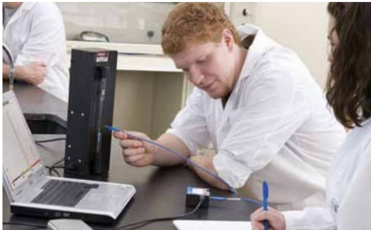
Examining the spectrum from a Helium gas discharge tube
