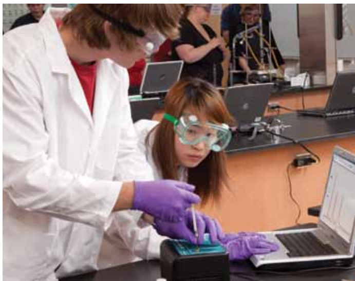
Students analyzing ketones using the Vernier Mini GC and a computer running Logger Pro
