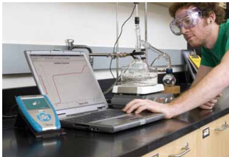
Conducting a distillation using LabQuest and the NEW Wide-Range Temperature Probe
