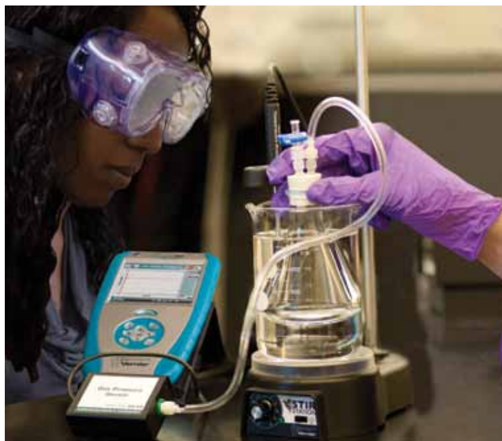
Measuring vapor pressure using LabQuest and a Gas Pressure Sensor
