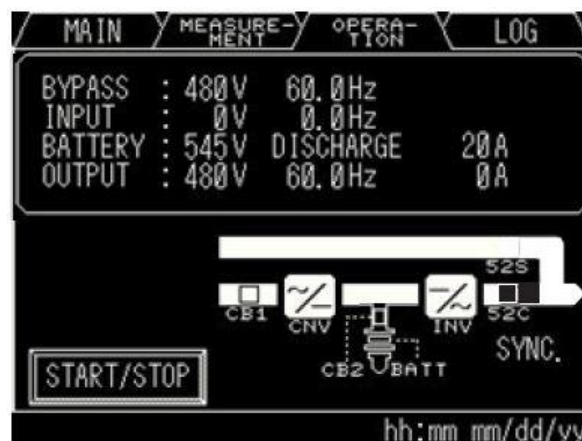
Figure 5-27 Open Battery Breaker
