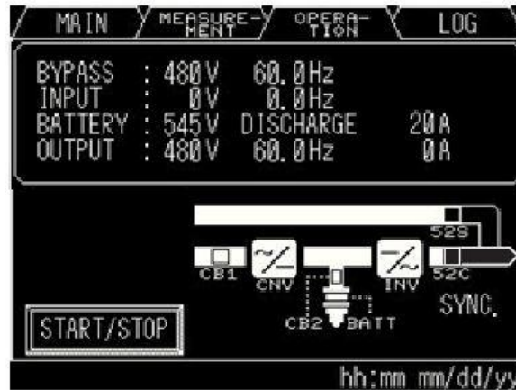
Figure 5-21 Close Battery Breaker
