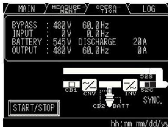
Figure 5-26 UPS Transfers to Bypass
