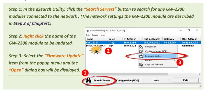
Step 4: In the "Open" dialog box, select the firmware file (GW2200.dat) that will be used to update the module and then click the "Open" button.
