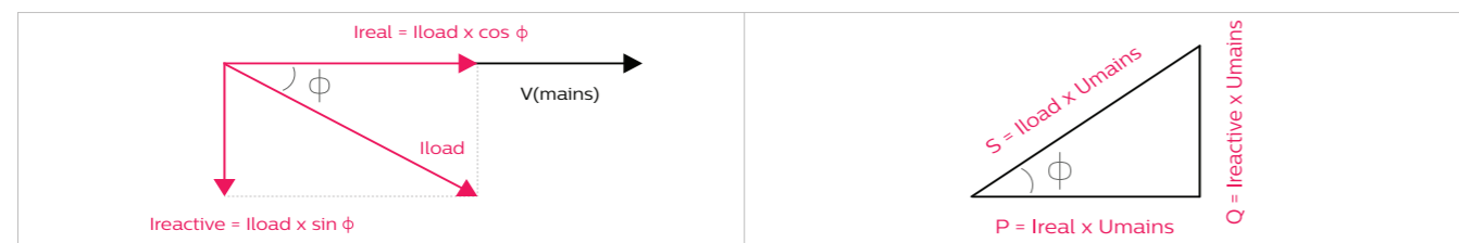
Figure 5: A: current decomposition, B: power triangle
