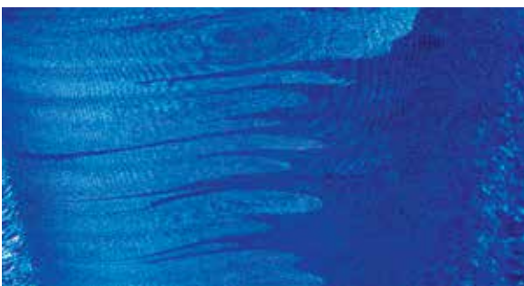
7075 and 6061 Aluminum Weld, etched with Barker's reagent, mag. 50x, polarized light ~Matthew Ryder and Xiangbin Wang; Worcester Polytechnic Institute; iMdc, Worcester, MA USA
