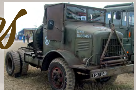
This International H-542, built for towing semi-trailers is a rare machine in the UK. They were assembled by International, Kenworth and Marmon-Herrington
