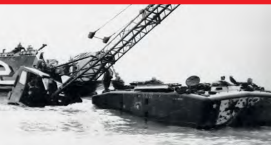
Company A, 1st AmTrac, landed in Vietnam on May 7, 1965. During the landing, as was routine, shore cranes 2N were used to unload wheeled vehicles and stores from landing craft. Here one is seen being recovered from the surf by an LVTP-5A1 (FRALEY / 26403921)
