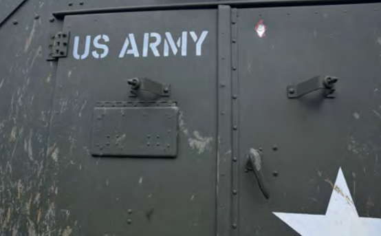
The troop/cargo bay has a simple rear door for loading and unloading
