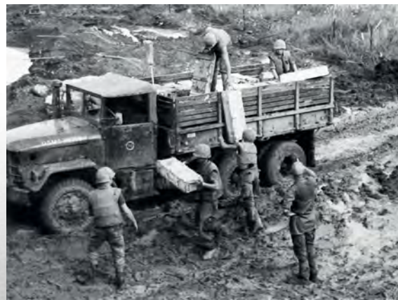
RIGHT: These artillerymen of 3rd Marine Division are unloading empty ammunition crates from an M35 series two and a half ton truck on December 7, 1967. Note the raised air intake forward of the cab on the right-hand side; this may indicate that the truck is fitted for deep wading. Note also the besom behind the cab for use in sweeping clean the load bed (PRIVATE FIRST CLASS O MCDOWALL / 26403701)
