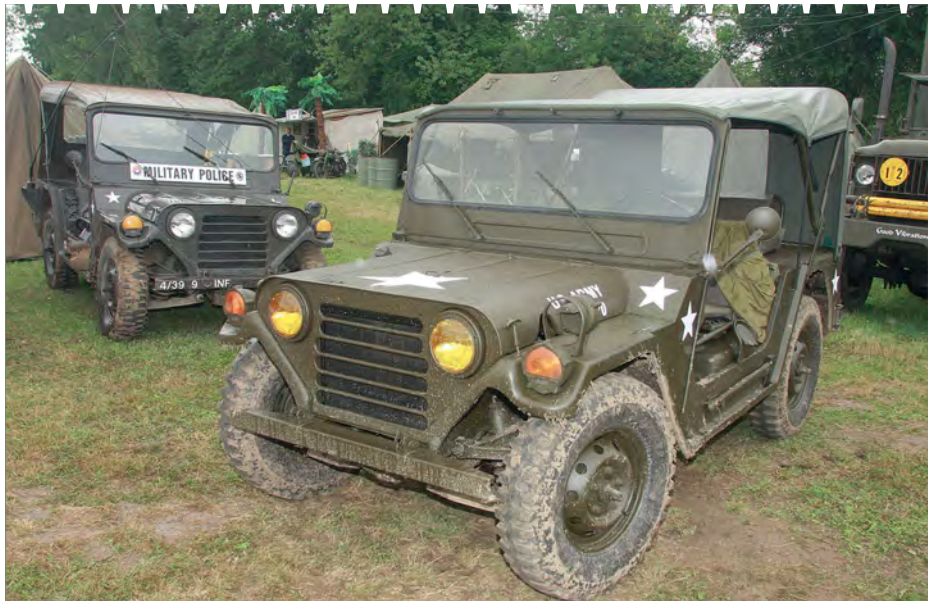
The M151A2, introduced in 1970, was a revised version of the M151A1 that incorporated redesigned suspension to reduce rollover accidents
