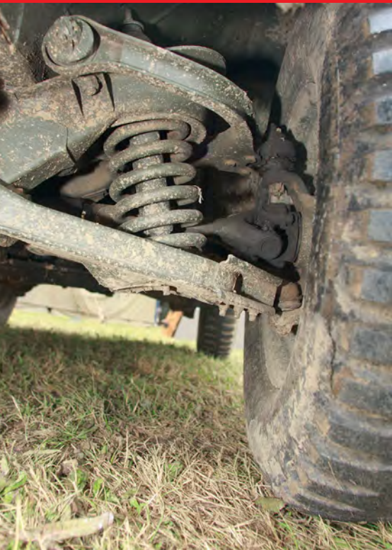
All versions of the M151 have independent front and rear suspension
