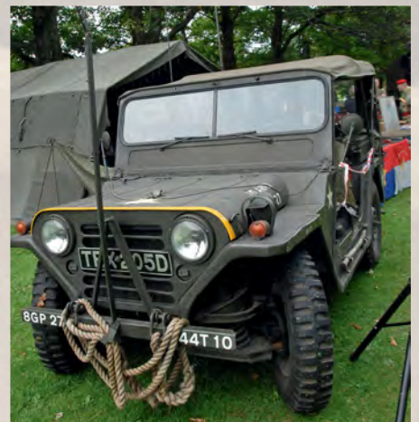
Roger Jerram's Truck, Utility, 1/4-Ton, 4x4, M151A1 also known as a 'MUTT' is part of his Vietnam period vehicle pool
