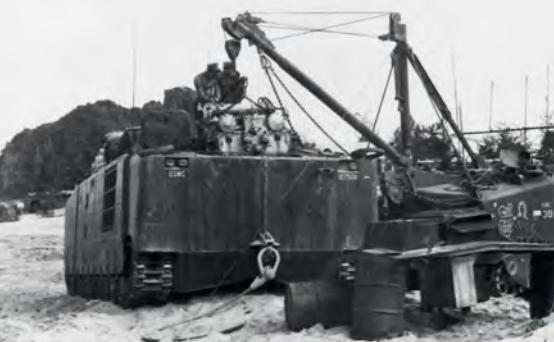
An LVTR-1 of Company B, 3rd AmTrac, changes the engine/transmission assembly of an LVTP-5A1 (CASSELLE / 26404125)
