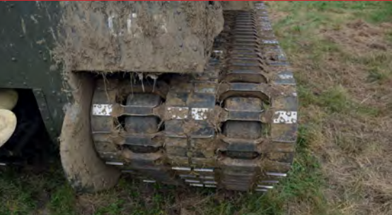
With traditional clutch-type steering, one track is slowed allowing the faster track to pivot the vehicle in the desired direction
