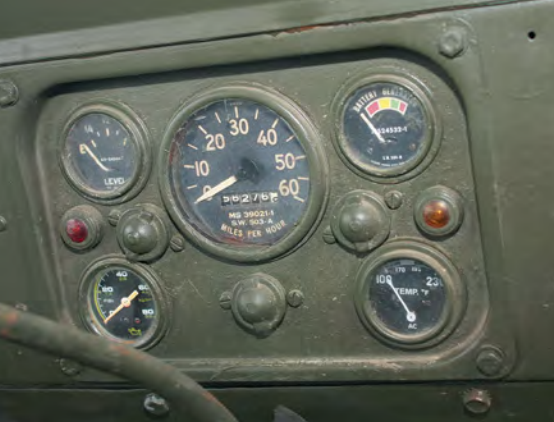
Five gauges in the dash is inherited from the Jeeps that preceded the M151
