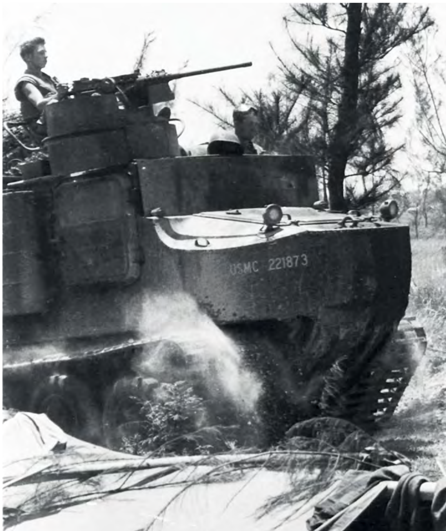
Operation Saline was developed into Operation Napoleon - Saline in May 1968. This Otter is moving forward in support of 2nd Battalion, 4th Marines in fighting east of Dong Ha; it has armour plate over the windscreen and round the ring mount (LANCE CORPORAL TEACHER / 26404143)
