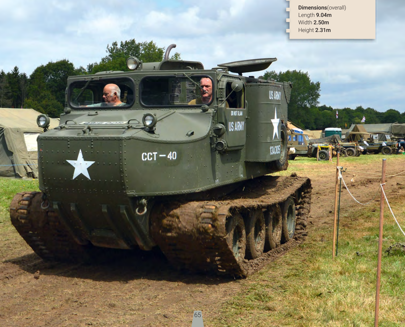
ABOVE: It is thought that there are fewer than ten fully operational M76 Otters in the world ABOVE LEFT: The tracks were an evolution of the type found on the Weasel, a single long rubber band with added metal cleats and thicker rubber blocks BELOW: A 70 gallon fuel capacity gave a approximate 200 mile road range
