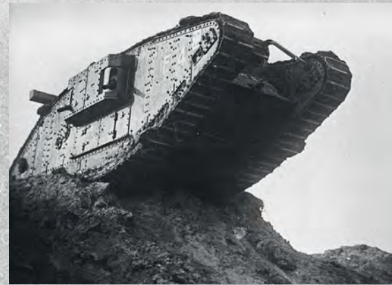
On the rear of 'Flirt II' is the large unditching beam which was chained to both tracks and which would help extract the tank if it became stuck (PHOTO BOVINGTON TANK MUSEUM)
