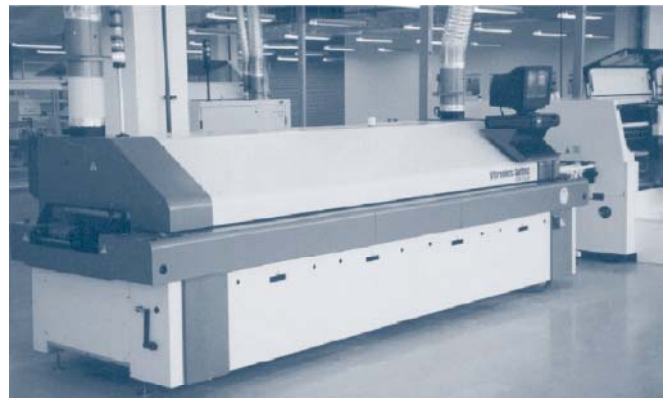
The Vitronics reflow oven has eight heating and two cooling zones and is the last step in the SMT process.
