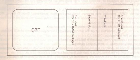
\* Although the fourth slot is provided for a ROM package (to use a ROM package, it must be inserted into this slot), a RAM package may be inserted into this slot to increase RAM area. The fourth slot can be used for either a RAM or a ROM package.
