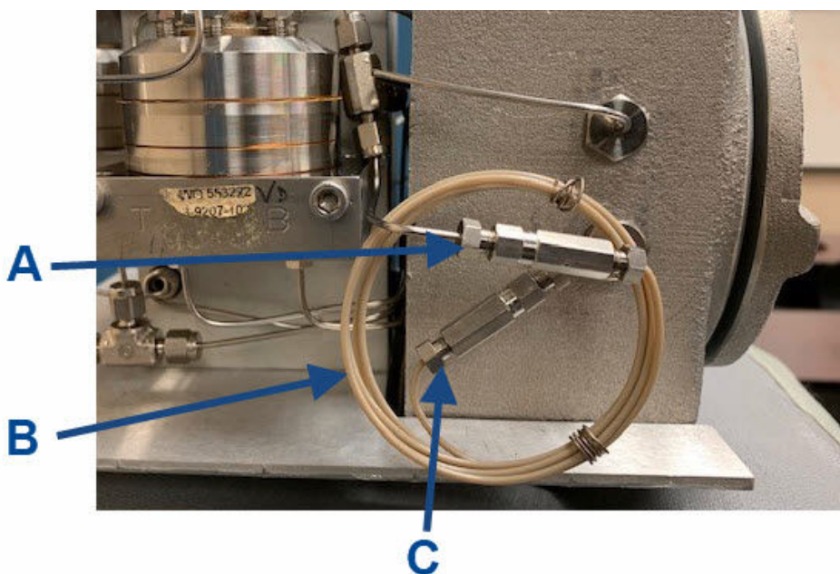
Figure 2-3: New 10-ft. (3 m) Restrictor (R2)
