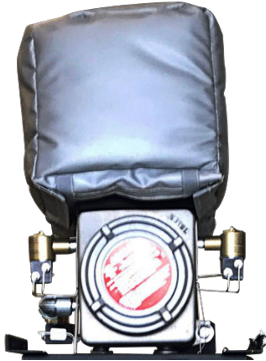
Figure 2-5: Upper Enclosure Insulation Cover
