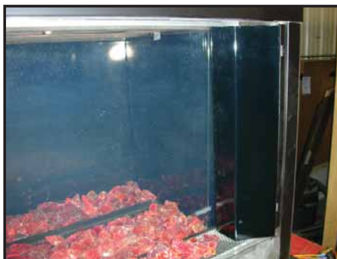
Figure 10. Outside Corner Trim Piece Installed.
