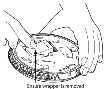
The backing plate has a safety mechanism which prevents the alarm being installed without a battery. When the battery is inserted this safety mechanism is released meaning that the alarm can be attached to the backing plate.
