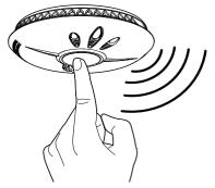
**a** Press and release the test/silence button, the alarm sound will shortly stop and the Escape Light will switch off.
