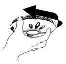
**a** Remove the alarm from its mounting plate by turning anti-clockwise
