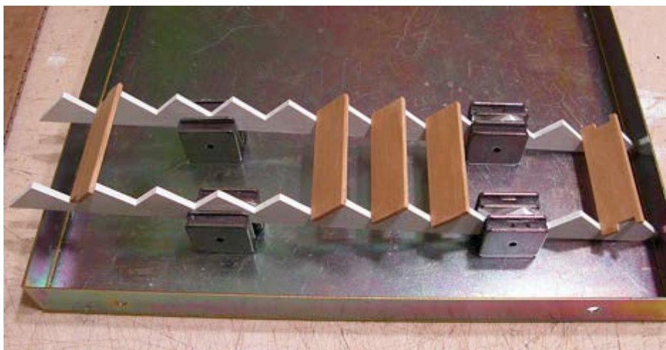
As can be seen by this example the tread project past open cut stringers.
