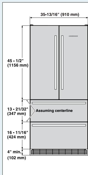
When installing CS 20 units into a row of cabinets or wall units, use these dimensions to achieve a custom look with the cabinetry.
