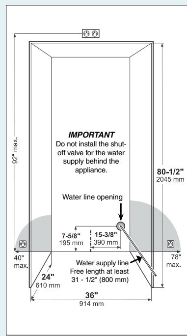
The position of the electrical outlet can be within the grey shaded areas or above the appliance.
